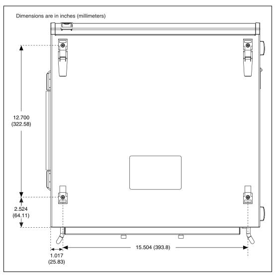
Figure A-2. NI PXIe-1065 Chassis Dimensions (Bottom)
